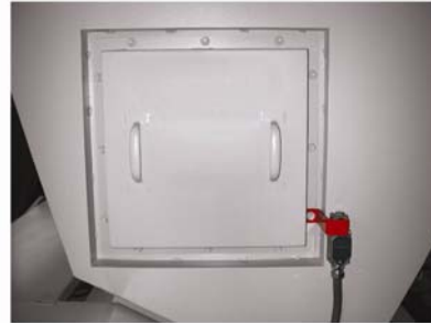
Side cleanout door with safety interlock
