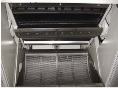
Tangential feed cutting chamber allowing for better ingestion of feedstock
