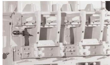
Drop down screen cradle for access during knife change and cleanout
