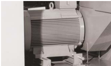
Outboard mounted motor with "heavy duty" flywheel
