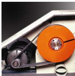
Heavy solid flywheel for added inertia
