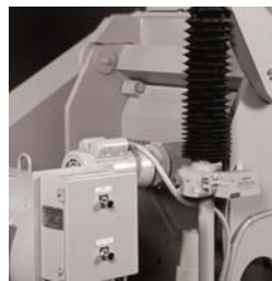
Clam shell opening with mechanical screw jack
