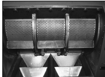
Standard tangential cutting chamber can be modified for bed knife placement to suit changing and demanding production requirements
