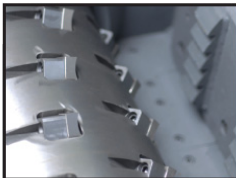
Large diameter rotor with "swing style" ram and serrated front plate.
