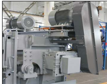
Dual drive motors with heavy-duty self-aligning gear box maximizes torque for high throughput shredding with reduced noise levels.
