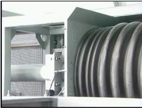
Telescoping ram provides positive pressure to pipe to ensure constant throughput.
