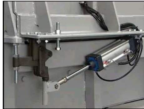
Automatic locks with light curtains provide redundant safety throughout the loading and feeding cycles.
